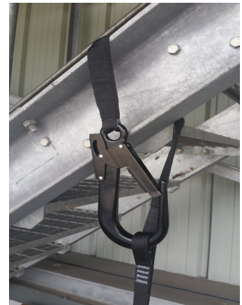
Large loop back facility
